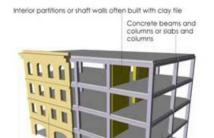
Multi-wythed brick masonry exterior one or more wythes built within the column/beam envelope as infill
