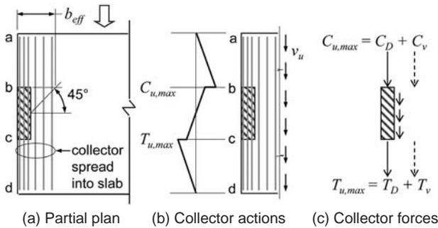
**Figure 6-6** – Force transfer where a collector is wider than the vertical element to which it transmits diaphragm shears. Note that the collector force might not be zero at the “free” end if there is lumped mass due to cladding or other perimeter elements.
