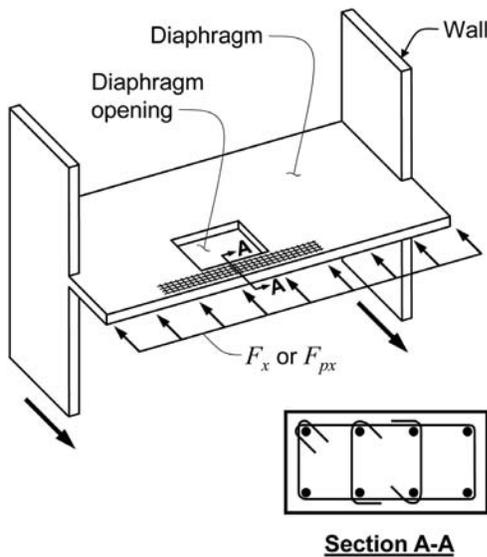
Figure 7-1 – Confinement reinforcement in axial struts around openings.
