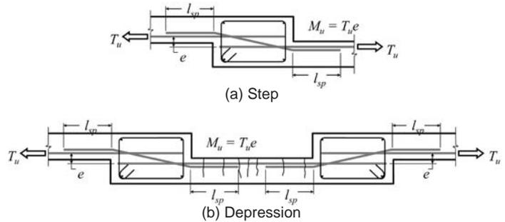
**Figure 7-5** – Steps and depressions. (b) shows flexural cracking of the depression that could be induced by the eccentric loading.
