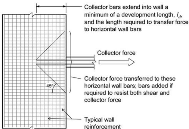
**Figure 6-8** – Transfer of collector force directly to shear wall.
