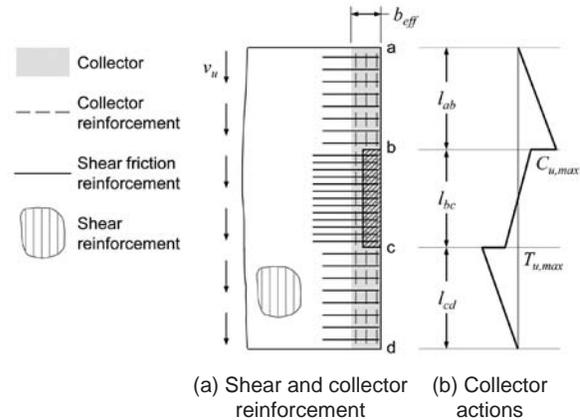
Figure 7-2 – Shear reinforcement, collector reinforcement, and shear-friction reinforcement.
