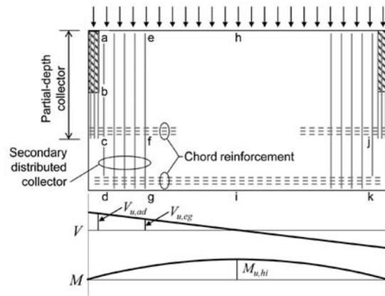
**Figure 6-7** – Partial-depth collector.
