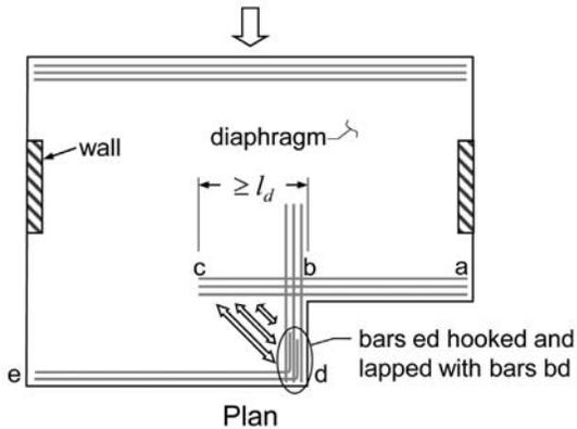
**Figure 7-4** – Reinforcement associated with re-entrant corners.
