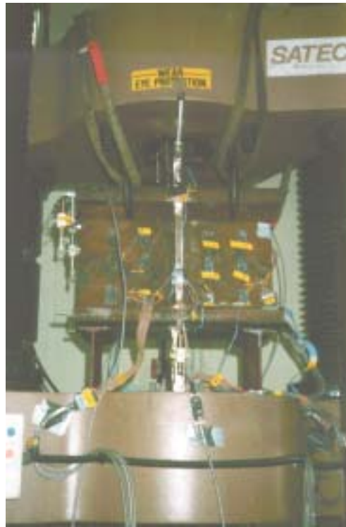
Figure 5-7 Typical Tee-Joint Test Setup in the 2670 kN Capacity Universal Testing Machine Showing Location of Strain Gages and LVDTs
