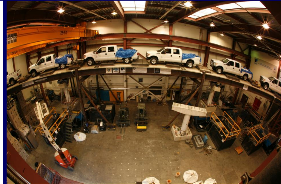
Six F250 trucks on bridge model (fish-eye view)
