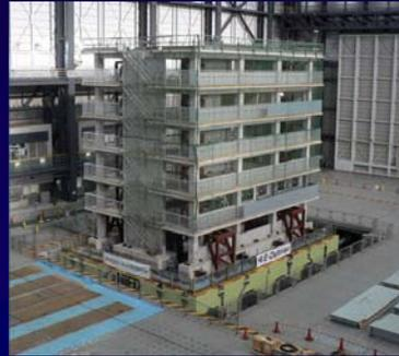
Full-scale earthquake simulation test on reinforced concrete building structure using E-Defense on January 2006. The test was part of five-year national research project - DaiDaiToku. The specimen was a 6-story wall-frame structure, 2 by 3 bays. NSF has agreement w/MEXT and NEESInc has agreement w/NIED for joint utilization of NEES and E-Defense facilities.
