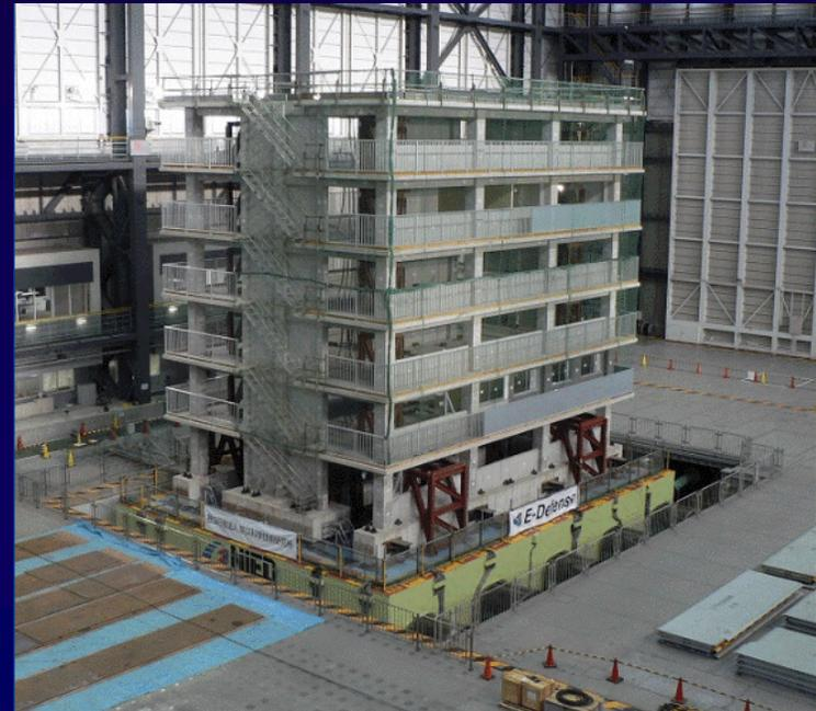
Full-scale earthquake simulation test on reinforced concrete building structure using E-Defense on January 2006. The test was part of five-year national research project - DaiDaiToku. The specimen was a 6-story wall-frame structure, 2 by 3 bays. NSF has agreement w/MEXT and NEESinc has agreement w/NIED for joint utilization of NEES and E-Defense facilities.
