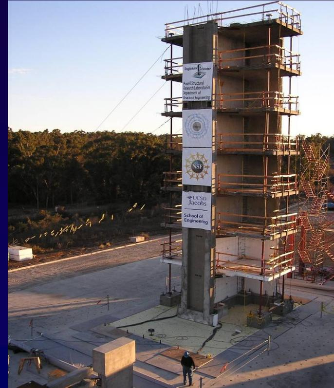
7-story reinforced concrete building test at UCSD NEES outdoor shake table showed that a structural wall with half the amount of reinforcing steel required by most building codes, but with more optimal layout, can better resist seismic loads.
