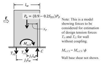
Figure 5-1 – Model for initial selection of flexural tension reinforcement.
