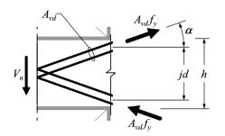
Figure 5-15 – Free-body diagram of half-span of a diagonally reinforced coupling beam. (Gravity loads not shown.)
