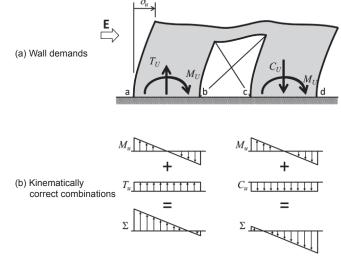
Figure 5-8 – Elevation of laterally displaced coupled wall system.
