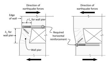
Figure 5-10 – Reinforcement required above and below wall pier.
