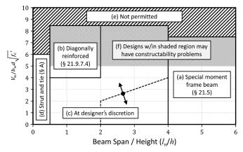
Figure 5-11 – Seismic coupling beam design space.
