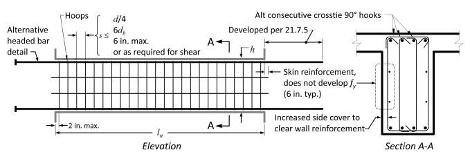
Figure 5-12 – Details for conventionally reinforced coupling beams.
