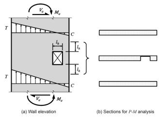
**Figure 5-18** – *P*-*M* analysis at irregular opening.
