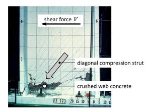
Figure 3-4 – Web crushing due to high shear force in laboratory test.
