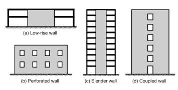
Figure 2-1 – Some illustrative structural wall elevations.
