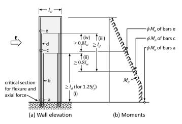
**Figure 5-9** – Bar cutoffs for vertical reinforcement for idealized  $M_u$  moment diagram.
