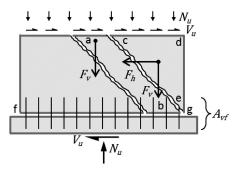
Figure 3-6 – Shear yielding and shear sliding in a squat wall.
