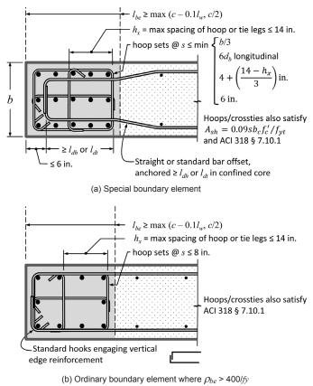
Figure 5-3 – Special and ordinary boundary elements.
