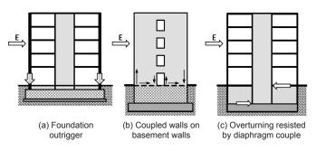
Figure 2-6 – Various ways to spread overturning resistance.
