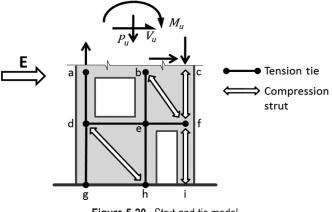
Figure 5-20- Strut-and-tie model.
