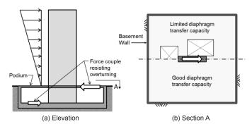
Figure 2-5 – Force transfers between walls and diaphragms.
