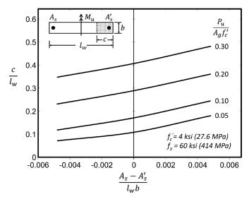
**Figure 5-2** – Approximate flexural compression depth. For flanged sections, adjust *A<sub>s</sub>*, *A'<sub>s</sub>*, and *b* considering effective flange width.
