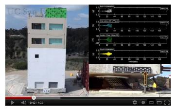
Excerpt from <u>video on BNCS test</u> conducted in April 2012. Left side shows test building on UCSD shake table. Upper right shows instruments tracking motion parameters captured by building sensors. Lower right shows base isolator flexing under the building (vertical arrow measures lateral movements). Courtesy of BNCS Project Core Team.
