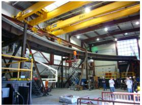
0.4-scale curved highway bridge model tested recently on shake tables in the Large-Scale Structures Laboratory at the University of Nevada, Reno (UNR) NEES equipment site. Courtesy of UNR Department of Civil and Environmental Engineering.
