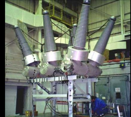
PEER support for IEEE 693 – Recommended Practice for Seismic Design of Substations
